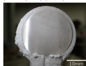
1-inch Ga 2 O 3 epitaxial wafer grown by the oxide vapor phase epitaxy (OVPE) method
