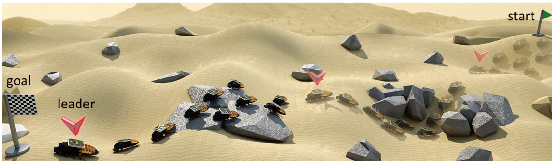
Illustration of cyborg insects moving as a swarm under the guidance of a leader cyborg insect
