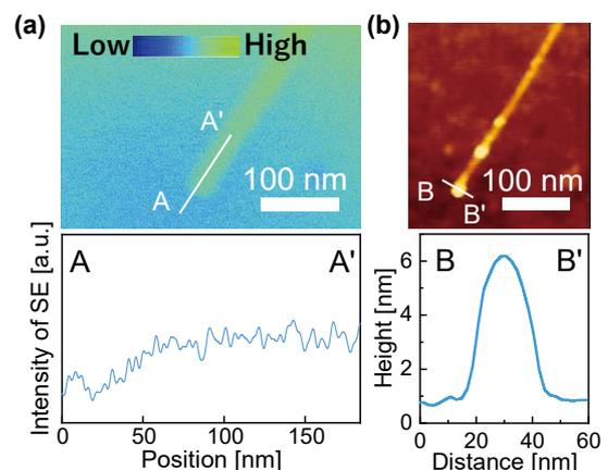
Figure 3 (a) Secondary electron yield map and (b) atomic force microscopy image of an aligned CNT tip.
