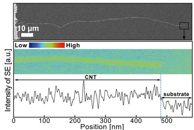
Figure 2 Scanning electron microscopy image and secondary electron yield map of an aligned CNT grown from nanodiamond.
