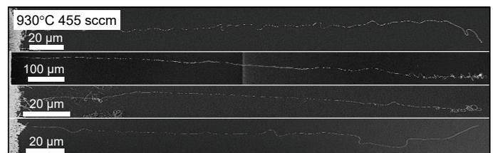
Figure 1 Scanning electron microscopy images of aligned CNTs grown from nanodiamond.
