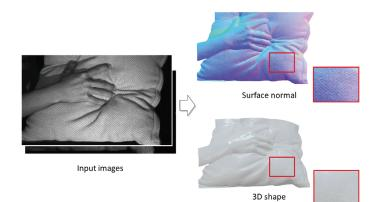
Figure 3: 3D reconstruction of a dynamic scene
