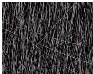
SEM image of poly( \epsilon -caprolactone) (PCL)-based electrospun scaffold
