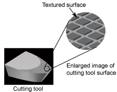
Fig. 1 Concept of the textured cutting tool
