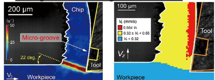
Fig. 3 Material flow in the vicinity of the cutting point
