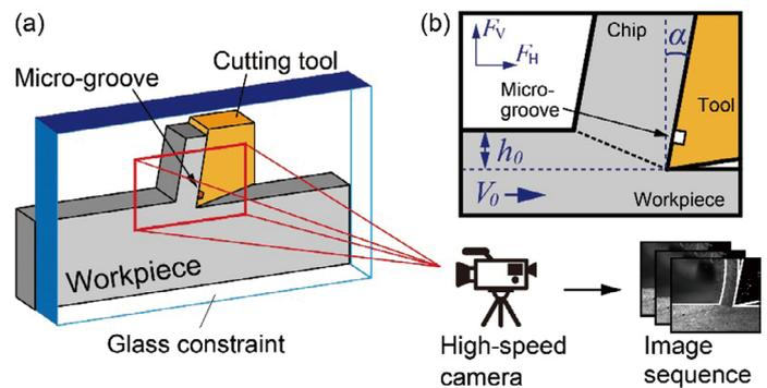
Fig. 2 In-situ observation of the metal cutting process
