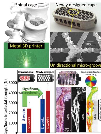
Figure 1. Titanium alloy spinal cage with a micro-groove structure based on the precise shape control capability of a metal 3D printer. The micro-groove structure induces mechanically integrated high quality bone, resulting in a significant increase in strength at the initial implantation period compared to conventional cages.
