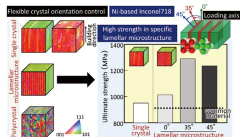
Figure 2. Flexible control of crystallographic texture achieved via metal 3D printer, and unusual strengthening by forming a specific lamellar structure (example of Inconel 718). Further strengthening is achieved by changing the resistance to slip deformation at the layer interface by changing the loading axis.
