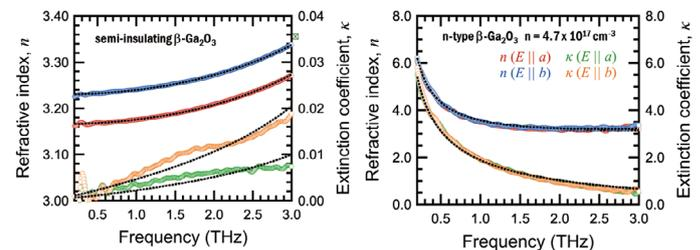
Refractive index spectra for wide bandgap semiconductor of  $\beta$ -Ga<sub>2</sub>O<sub>3</sub> in Terahertz range
