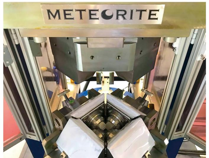
Multi-anvil-type high-pressure apparatus.
