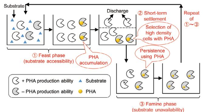
Principle of the aerobic dynamic discharge process applied for rapid enrichment of PHA-accumulating bacteria from WAS
