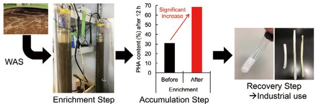
Flow of PHA production using WAS as the biocatalyst
