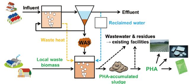
Concept of evolving a wastewater treatment plant as the bio-refinery to produce PHA
