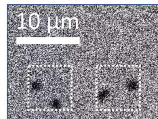
Figure 2 Skyrmion pair confined in square cells. Skyrmions interact with each other through magnetic dipole interaction, and information is propagated.
