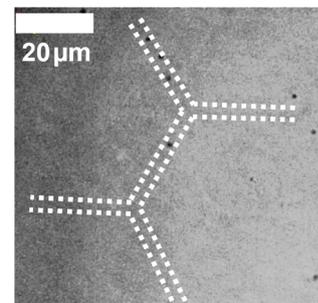
Figure 1 Circuit of skyrmions in Brownian motion. The black dots are skyrmions, which move randomly in the circuit without external energy supply.
