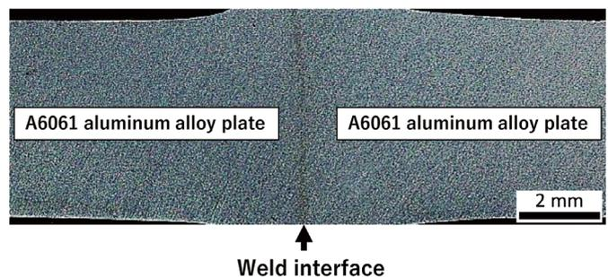
Fig. Cross sectional image of A6061/A6061 weld interface. Very thin weld interface is formed between two aluminum plates.
