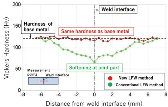
Fig. Hardness distribution of Al6061-T6 joints. Formation of softening region can be completely suppressed by new LFW method.
