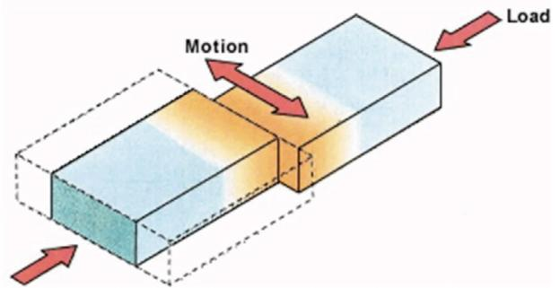
Fig. Schematic drawing of LFW. In linear friction welding, a softened flash is discharged from a welding interface to form a new surface to accomplish the welding.
