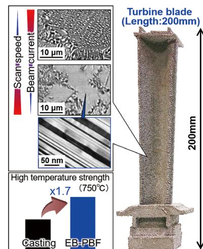
Fig. 2 It is possible to control microstructure of TiAl alloys by EB-PBF. A nano-scaled layered microstructure can be obtained through a unique phase transformation. The strength of the alloys with the nano-scaled layered microstructure is 1.7 times higher than that of casting alloys.
