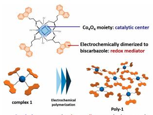
Catalytic center and redox mediator can be integrated via electrochemical polymerization
